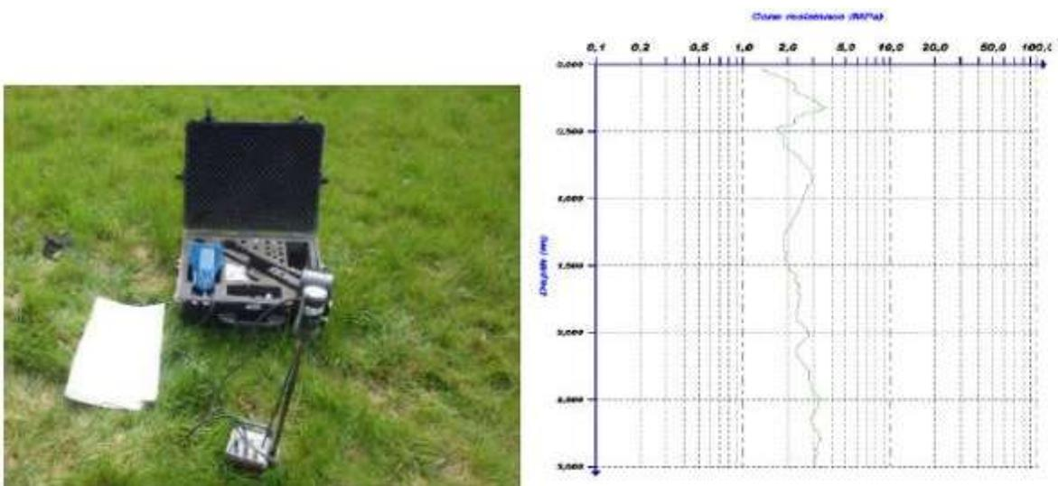
Fig. 4: Panda2 penetrometers and real penetrometer log
