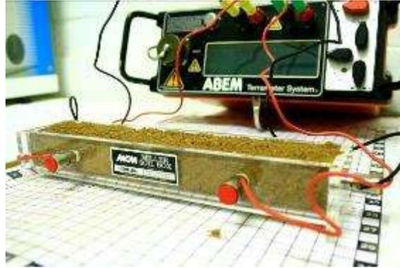
Picture 2: Soil-Box device for measurement of electrical resistivity in laboratory
