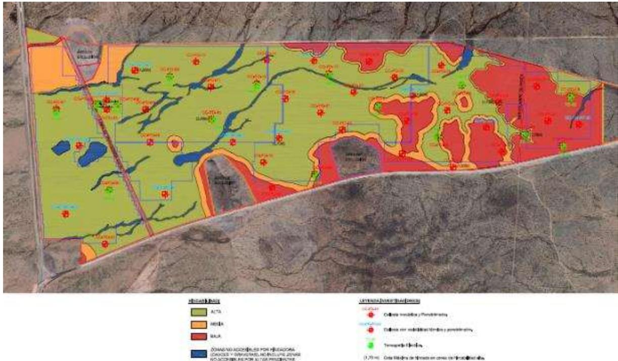
Fig. 2: Technical feasibility of driven piles drawing, developed by ORBIS TERRARUM
