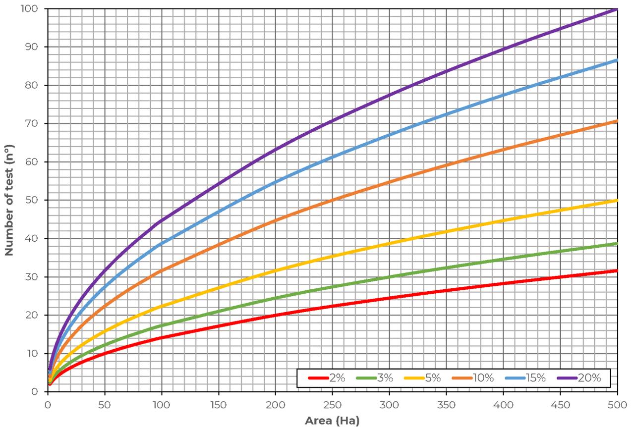
**Figure 4:** Number of test depending on the area to be investigated and its average slope.
