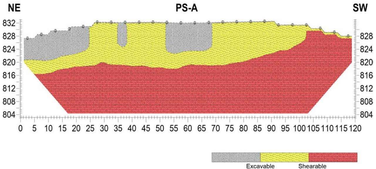
**Figure 6:** *Distribution of excavable, shearable and flyable areas of a P-wave velocity section.*
