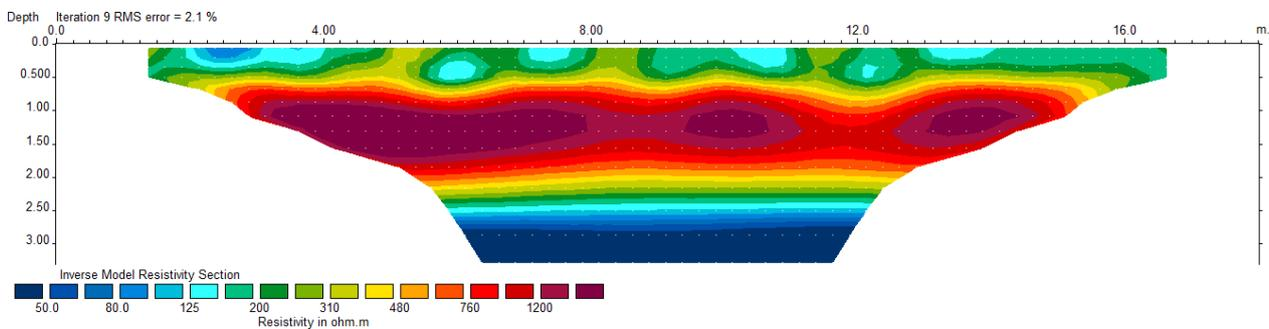
(c) Processed electrical resistivity section
