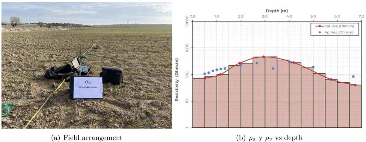
**Figure 2:** *Geoelectrical characterization by vertical electrical sounding test.*
