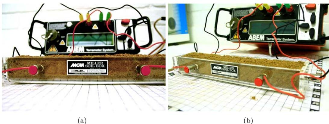
**Figure 3:** *Geoelectrical characterization through Soil-Box method.*
